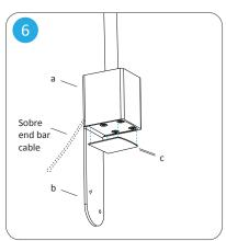
Attach the black adhesive to protect the screws.
