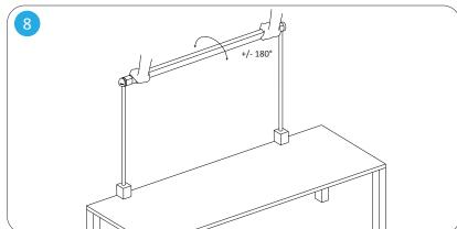
The luminaire can be turned 180 degrees each way to aim the light in the desired direction.
