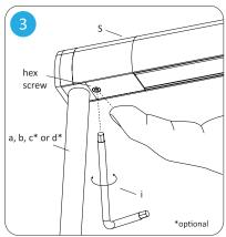
After the bars are fully inserted, push in the hex screw so it engages the end bars and the connecting bar(s). If the screw head shows above the surface, tighten the screw until it is flush with the surface using the provided hex key.
