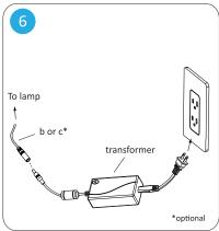
Connect the transformer to the lamp cable, then plug in the transformer to the wall outlet.
